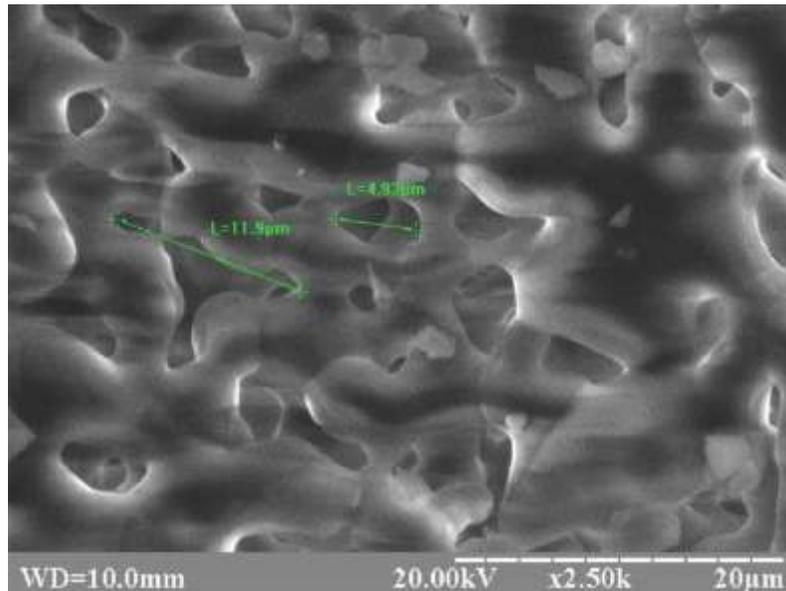
**Fig. 1: Microstructure of the Osteoplastic Material "ChronOS™". Visible Micropores of Size from the 4.93  $\mu\text{m}$  to 11.9  $\mu\text{m}$ . Electronic Scanning Image. X 2500.**
